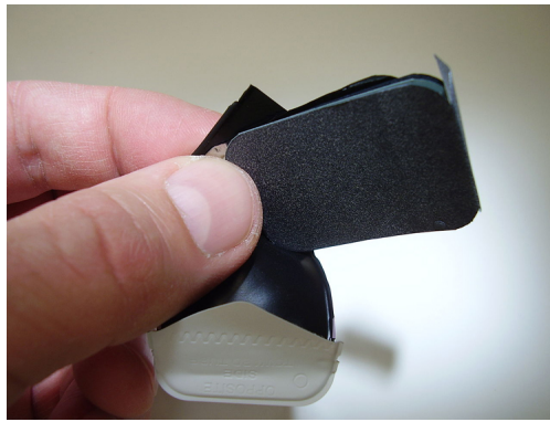
Figure 31.8 Film badges contain film similar to that used in dental x-ray film and is sandwiched between various absorbers to determine the penetrating ability of the radiation as well as the amount. (credit: Werneuchen, Wikimedia Commons)
